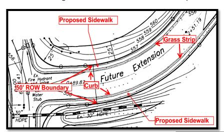
Plan view on sheet 5 of the Chadwick Estates approved plans. Specifically illustrates the curb line, 2' grass strip, sidewalk, and 50' ROW
